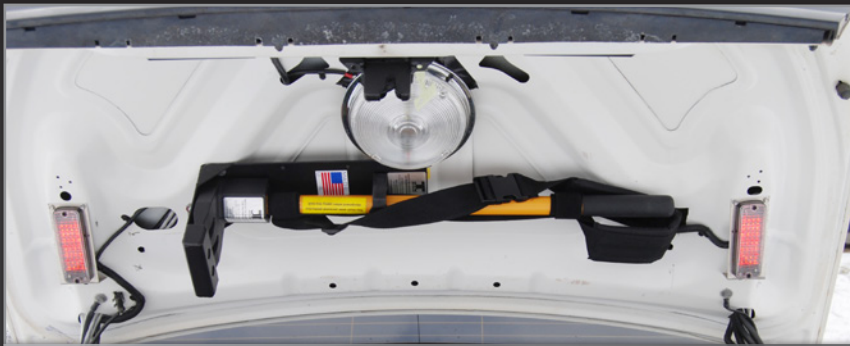
▲ The CLAW is easily mounted (teeth-protected) in either a vertical or horizontal position in a patrol vehicle. Grab the patrol rifle, grab the patrol CLAW, and go.
