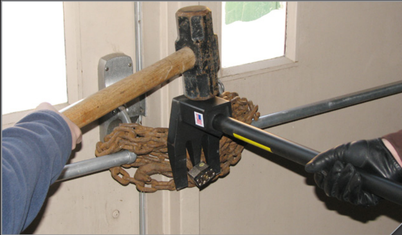
▲ Chain and padlocks are the latest Active Shooter trick. The CLAW can break locks, as well as remove hinges and deadbolts.
